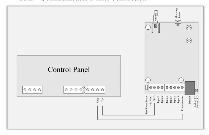
Radina Tau V5 has built-in communicator/dialer receiver. It can receive data from each security panel with communicator/dialer option. Settings for the security panel (in some models additional settings may also need to be made):
