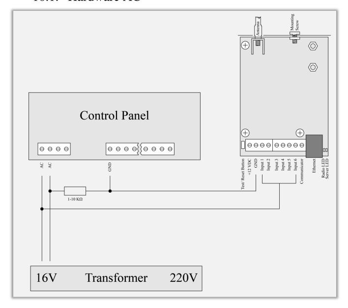
Each of the digital inputs could be used as a "Hardware AC" input. In this mode it will monitor the AC and generate a message for "AC Loss/AC Restore".
