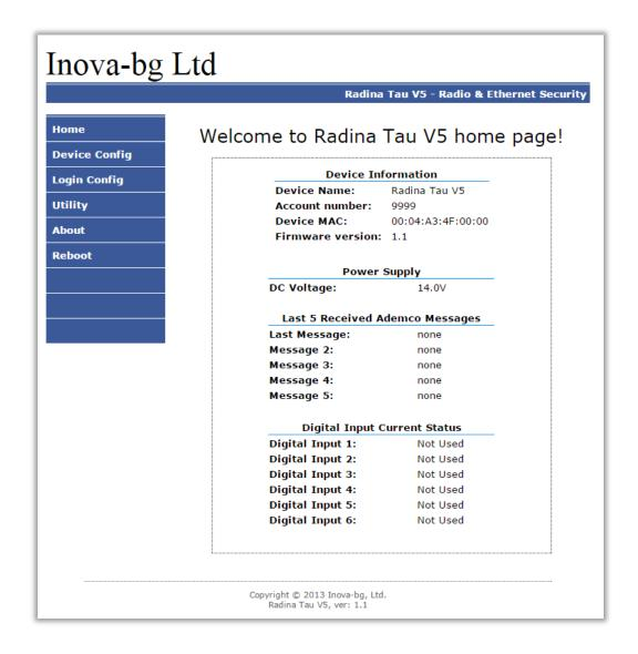
On the homepage you can find main information about the device, current status of the input voltage, last 5 messages received from the communicator and the current state of each digital input. Through the menu you could select one of the following actions:
