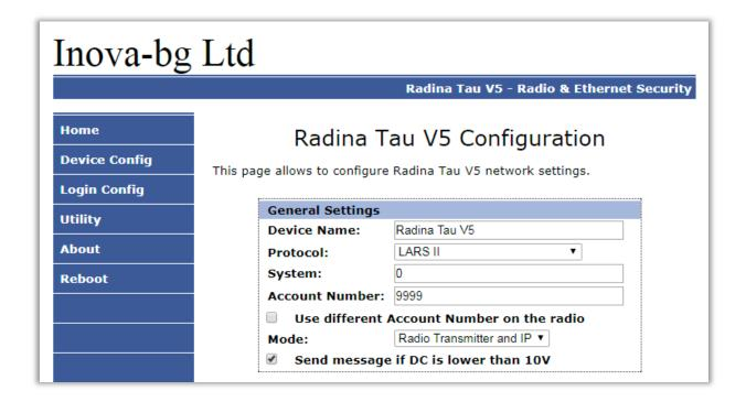
**Device Name** – Enter the name of the device. This value is used only for user convenience – to identify devices if you have more than one connected to one network. Maximum length -30 symbols.
